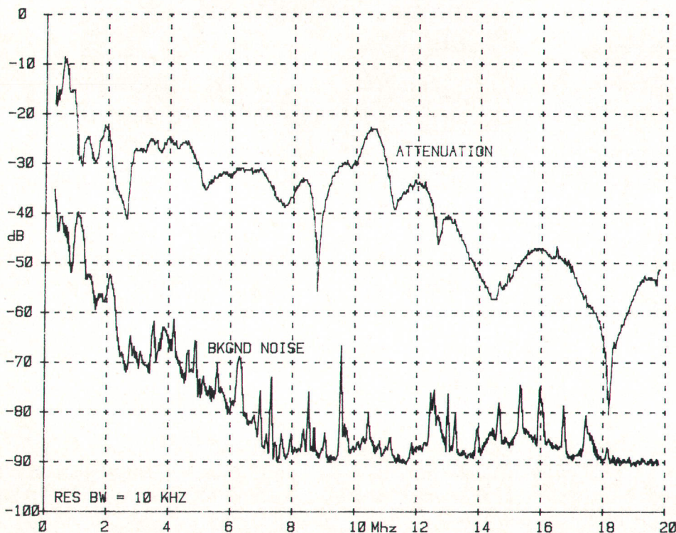
Fig. 1. Typical attenuation and background noise for a 100-foot-long power-line path (reference = 0 dBm, resolution bandwidth = 10 kHz).
