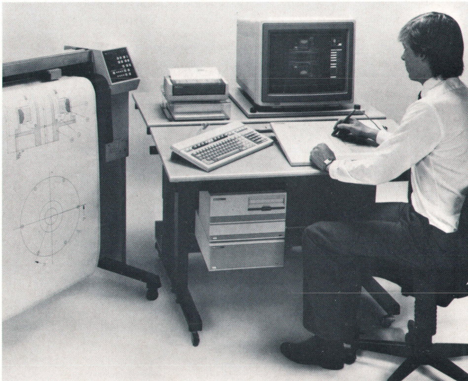
Fig. 1. The Mechanical Engineering Series 5 and Series 10 Workstations of HP's DesignCenter are versatile systems for two-dimensional drafting (Series 5 and Series 10) and mechanical design (Series 10) applications. Both feature a friendly and easy-to-learn user interface designed for technical illustrators, drafters, and engineers. The Series 5 provides many tools for the preparation of drawings, flowcharts, schematics, layouts, and documentation and can be easily upgraded to the Series 10, which provides many facilities for mechanical engineering design such as parametric design evaluations, customizability, and interfaces to other CAD systems (e.g., for finite-element analysis) and to numerically controlled (NC) machinery.
